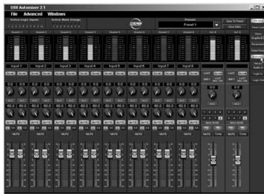
The DX8 Automix view includes an Automatic Level Control and a Gate control
