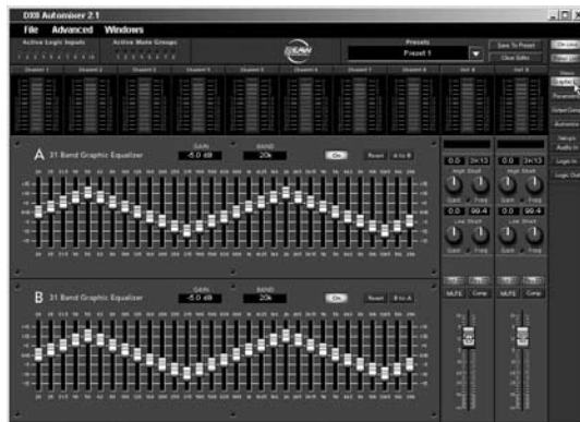
The DX8 Graphic EQ view offers 31 bands of control on ISO-centered frequencies for each of the two master outputs
