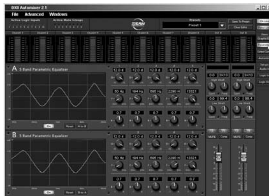
The DX8 Parametric EQ view includes 5 bands of control, as well as display windows that graphically represent the selected curves
